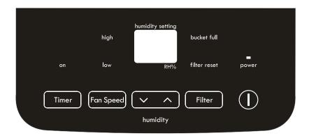
2. To turn the unit on, press the ON/OFF button. The unit will run in the factory setting of CONTINUOUS and high fan speed. In the Continuous Mode the unit will only display CO and not the room humidity. It is recommended you leave the unit running in the CONTINUOUS setting for the first three or four days until the sweating and dampness odors have stopped.
